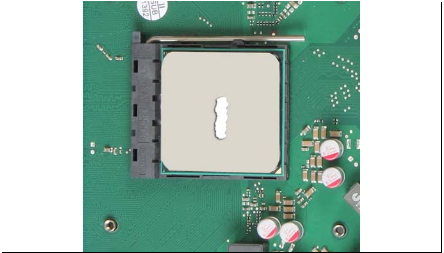
Figure 124: Applying thermal paste
